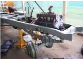
The remainder of the team (Peter Jarrett, Garry, & myself, plus Pete the welder on occasions, have progressively removed heaps of dirt/gunk & rust from the chassis & running gear, treated most of the chassis with
